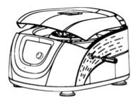
1) Open the lid: Use the included Door Key to press the button on the right side of the unit.
